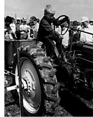
Figure 4.3.a. Oftentimes the youthful farm worker is willing to do more work than his or her mental and physical maturity will safely permit. Youth should never operate a tractor without a ROPS and seat belt.
